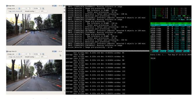
Autoware Object detection node running on Arm target. Using ArmNN and OpenCL backend for acceleration. This work is carried out by Eliot Lim (Arm). See the demo later in the demo area.
