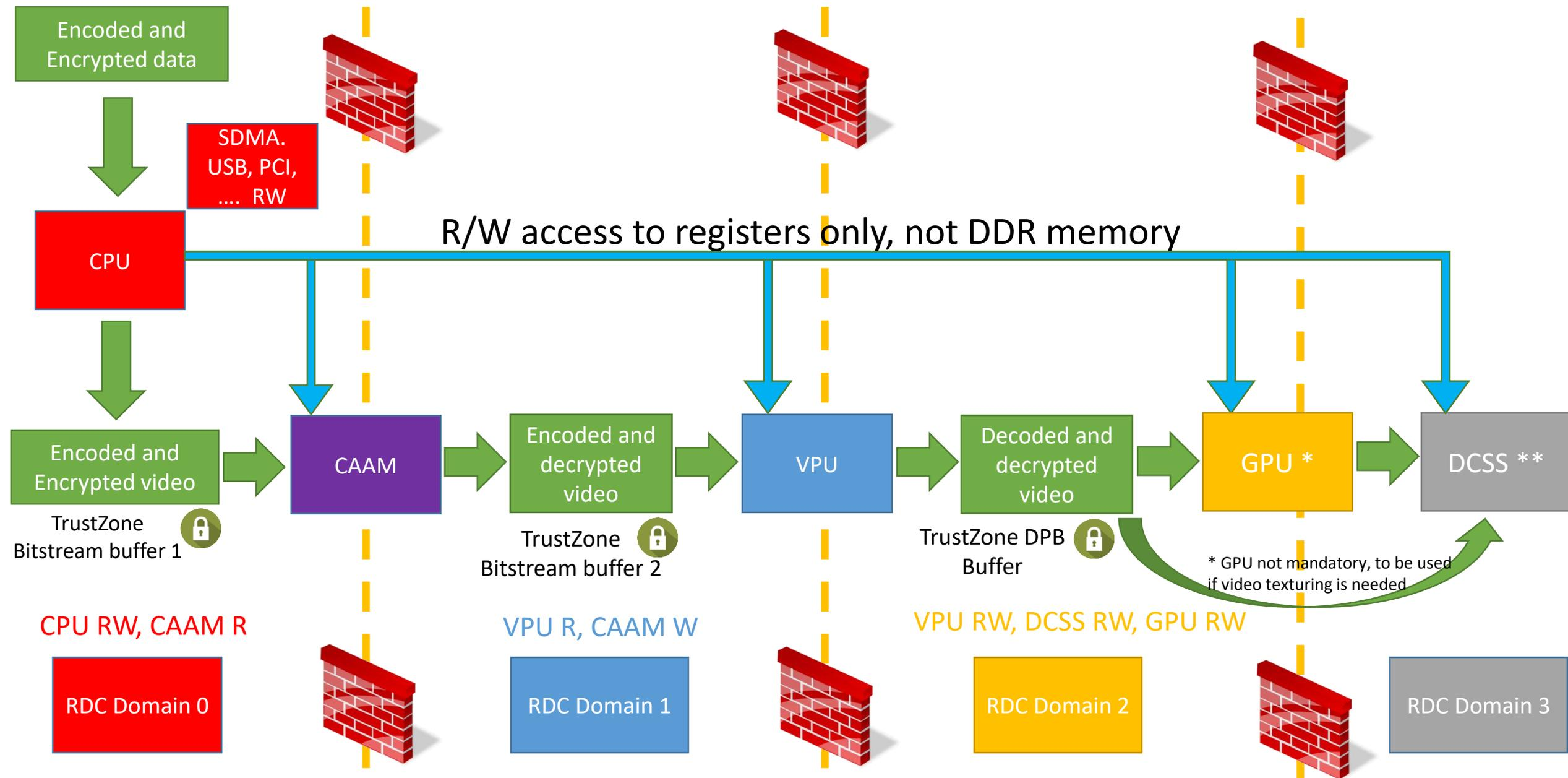
\*\* DCSS: Display Controller Sub System: to source up to three display buffers, on the fly composition (3 scalers, PIP) and drive display using HDMI 2.0a with HDCP 2.2
